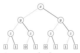
This tree is an ordered BBD (with variable order [x, y, z]) but is not reduced because transformations C1 and C2 are applicable.
