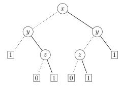
An application of transformation C1 followed by an application of transformation C3 produces the reduced OBDD
