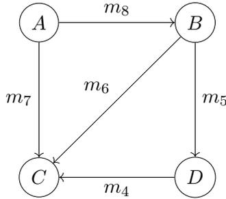
**Solution:** The start matrix would be  $N_0$ . The shortest distance matrix would be  $N_4$  where  $x_1 = \min(m_7, m_8 + m_6, m_8 + m_5 + m_4)$  and  $x_2 = \min(m_6, m_5 + m_4)$ . In matrix  $N_2$  and  $N_3$  we have  $x_3 = \min(m_7, m_8 + m_6)$ .
